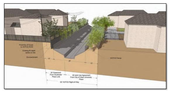
Figure 1-1: Cross-Section Depicting Constrained Portions of Poor Farm Ditch
