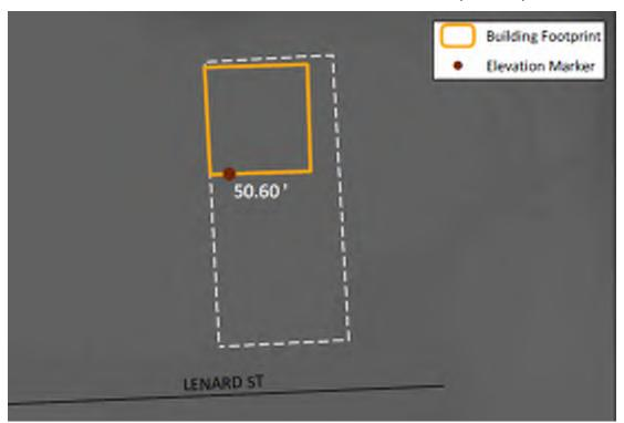
Figure 1. Illustrative example of first floor elevation calculation
