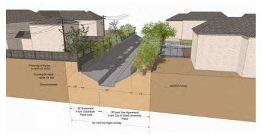
Figure 3 – Cross-Section Depicting Constrained Portions of Poor Farm Ditch
